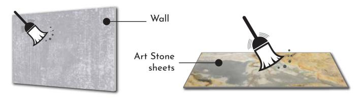
Cleaning walls and Art Stone sheets by broom, water or wipe. Make sure that all of surface are dry before doing next steps.
