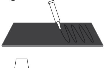
Applying glue directly from a tube or by notched trowel. The glue should be stretched full of stone sheet. With multi-component glue, should mix them before using.
